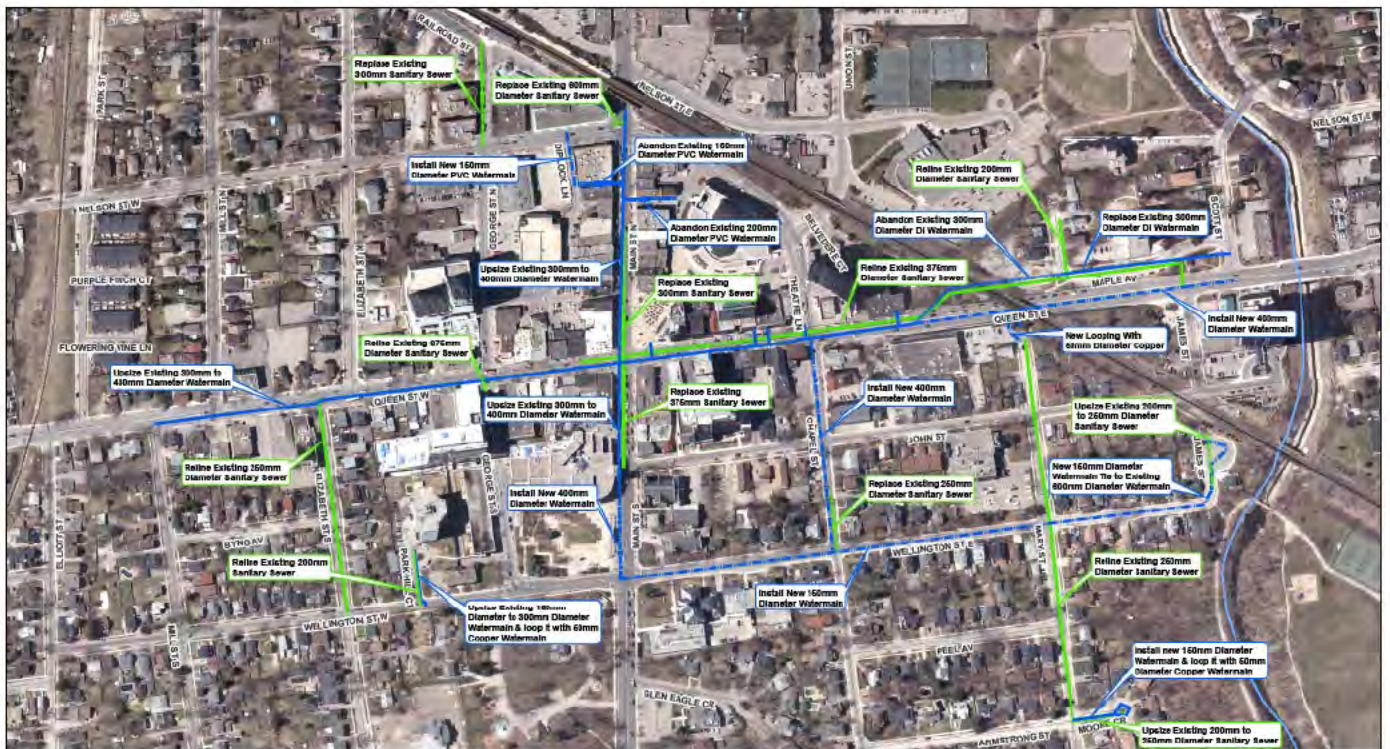
Region of Peel- Watermain And Sanitary Sewer Replacement/Relining Program For Brampton Downtown (Phase - 1)
